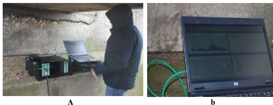
Fig. 5. 4 - Fig. 5. 4 - Determination of vibration values of the marine environment when sampling: a - an overview of the equipment used, b - recording the vibrations on the laptop screen
